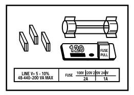
The line voltage selector board and fuse are located next to the power cord receptacle on the back of the analyzer.
