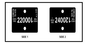
The board can be inserted in its slot so that any one of the four different voltage settings can be read from outside the unit.
